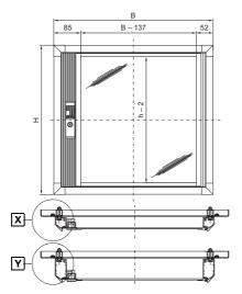
Viewing area (B -137) offset by 16.5 mm towards the hinge side
